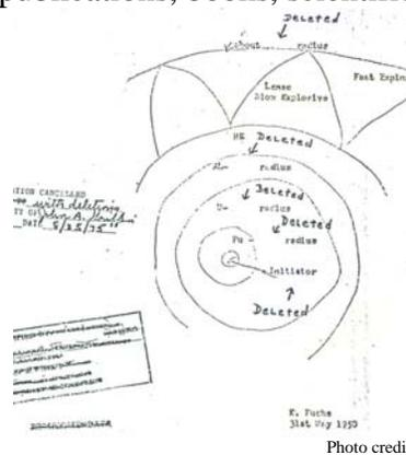
Fig. 1 K. Fuchs Drawing: Cross-section of Fat Man
